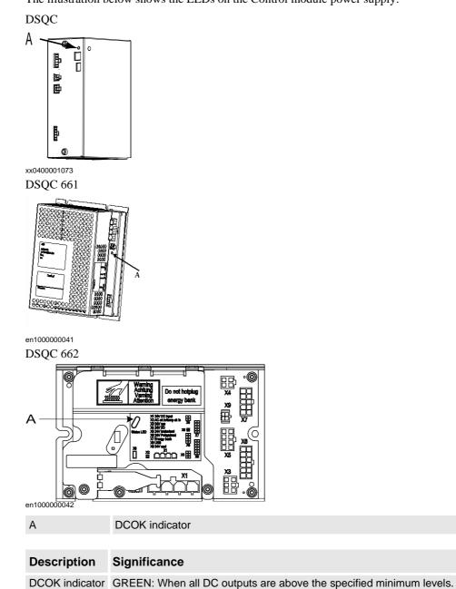
OFF: When one or more DC output/s below the specified minimum level.
