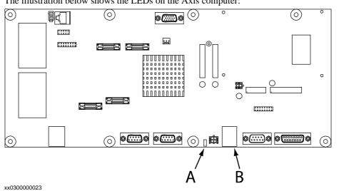
The illustration below shows the LEDs on the Axis computer:
