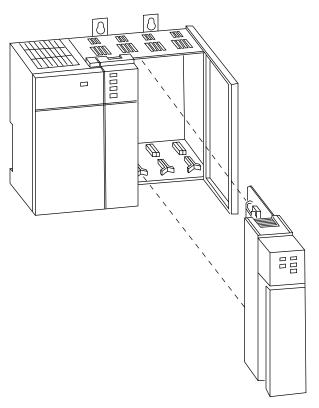
2. Slide your module into the chassis until both top and bottom retaining clips are secure. Apply firm even pressure on your module to attach it to its backplane connector. Never force your module into the slot.
