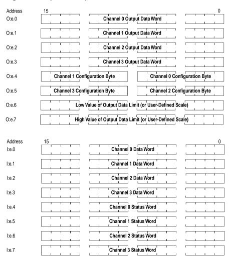
**Example** – If you want to reconfigure channel 2 on your module, and it is in slot 4 of the SLC chassis, you would modify the configuration word at address O:4.5. Alternatively, if you want to obtain the status of channel 2, you would check the status word at address I:4.6.
