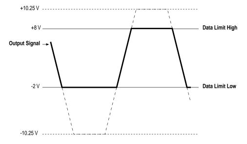
Note that whenever the requested output data values meet or attempt to exceed the output data limits, your module sets bits 10 or 11 in the channel status word to indicate a limit error. Note also that words 0 through 3 of the input image file (addresses I:e.0 through I:e.3) reflect the requested output data values and are not truncated.
